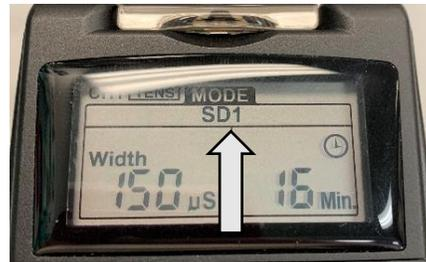
**6:** The Width is the full cycle of the wave pattern. To adjust the width of the wave pattern hit SET once and you will see width flashing on the screen. To increase or decrease the width press up or down on the arrows. The width of BodyMed Tens unit cannot be decreased below 50  $\mu$
